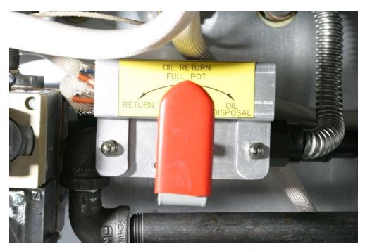
Turn the handle to the left to return oil from the filter pan to the frypot. Turn it to the right to discharge the oil to the disposal system.
